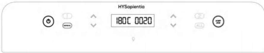
1. In the standby mode, press **MANUAL** to enter the Whole Compartment Custom Mode. The Whole Compartment Custom Mode is only applicable to the Whole Compartment Working Mode (the temperature sensing logic is consistent); The default temperature and time are 180 degrees for 20 minutes. Press the Start button to start running the set time and temperature. All the function keys at the bottom are off, only the light button remains.
