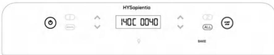
1. In the function selection, press (ALL) to enter the Whole Compartment Working Mode (In this mode, the right NTC acts as the temperature sensing NTC, and the left NTC does not participate in temperature sensing). All function keys at the bottom are enabled.
